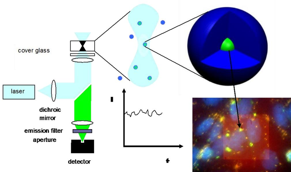
**Figure 1.** An FCS set-up used to characterize micelles, whose hydrophobic core is labeled by an organic fluorophore and a fluorescence microscopy image of mammalian cells, which have been exposed to an aqueous solution of these micelles.
