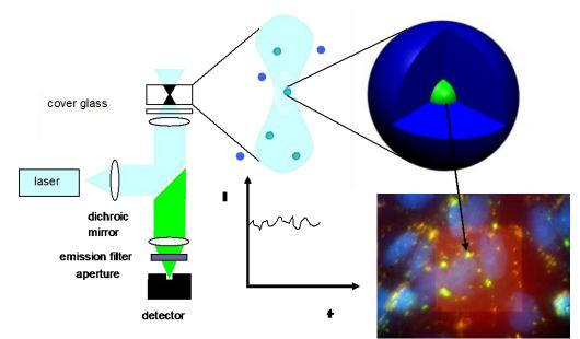
**Figure 1.** An FCS set-up used to characterize micelles, whose hydrophobic core is labeled by an organic fluorophore and a fluorescence microscopy image of mammalian cells, which have been exposed to an aqueous solution of these micelles.
